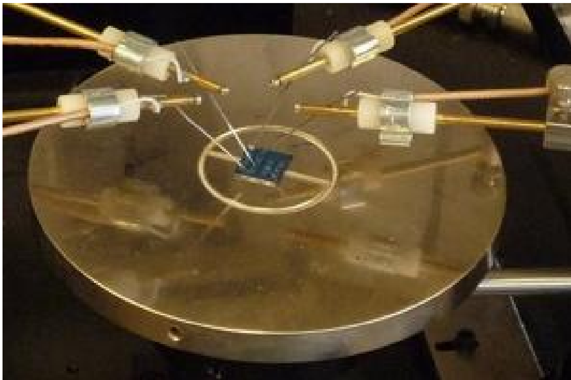
The organic circuit developed at the University of Washington that transmits positive and negative charges. Here it is undergoing a test. (Credit: Image courtesy of University of Washington)
